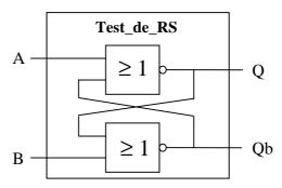
Entity test\_de\_rs is port (E1, E2 : IN bit; S1, S2 INOUT bit); end test\_de\_RS;
